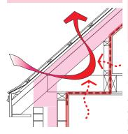
The thermal bypass occurs when the airtightness barrier does not follow the insulation.
